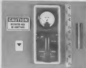
SOME OF the safety equipment used in radiographic inspection work are, from left to right, warning sign, film monitoring badge, survey rate meter, tape to identify radioactive material, and dosimeter.
